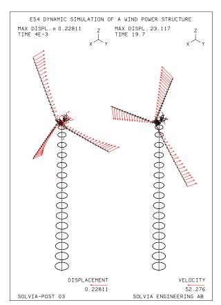
Vector plot of displacements at time 4 ms and of the velocities at time 19.7 s.
